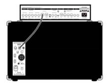
**MONO RIG** - Guitar processor (ex: Fractal Axe-FX Ultra) connected to the balanced XLR or ¼" unbalanced input (whichever is convenient) of the powered cab or wedge.
