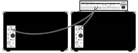
**STEREO RIG** - Connect the left and right outputs of a stereo processor to the inputs of two Reactors to create a wide, 3D sound.
