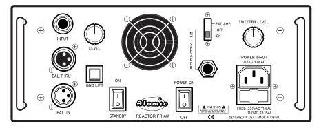
Figure 2 : Controls & Connections of the FR-AW Active Powered Wedge Model. The models have identical controls, described on the facing page.
